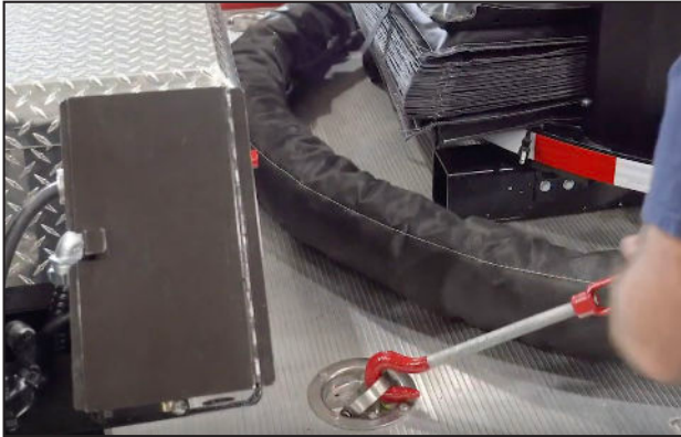
STEP 2.1: With back bar being tight, hook turnbuckle (side A) into streetside floor hook.
