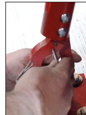
STEP 2.6: Place pins in bar hook eyelets to hold.
