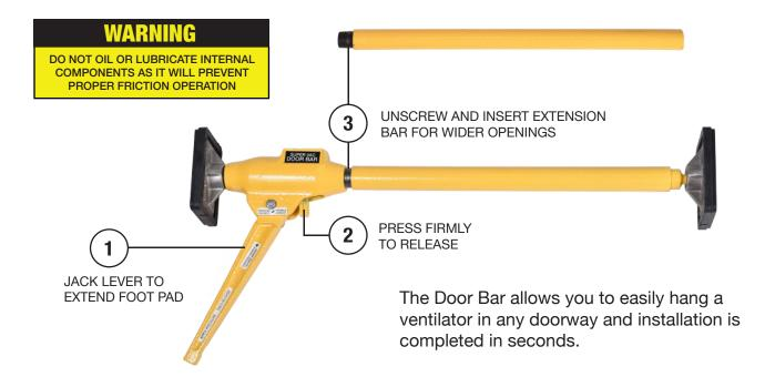
Door Bar is shipped partially assembled.
