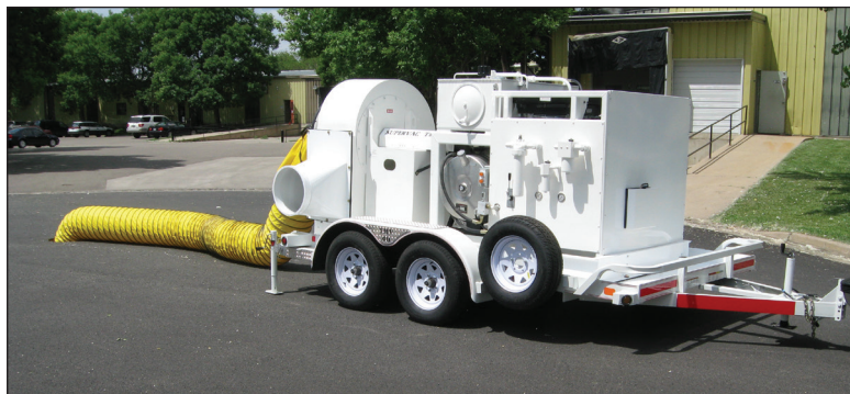
The TMV-40 was built to be mobile, run at a low decibel level and provide 15,000 cfm through an 18" x 25' duct at 5" static pressure.
